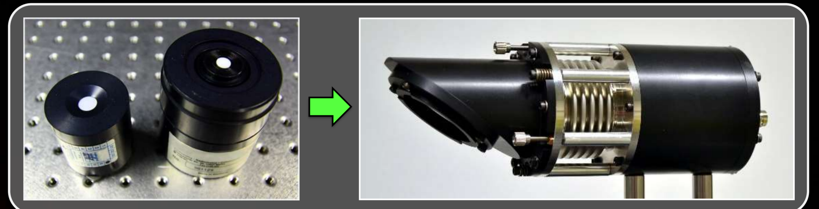
New Reference PQED-photometers without optical V(\lambda) -filters for NMIs
